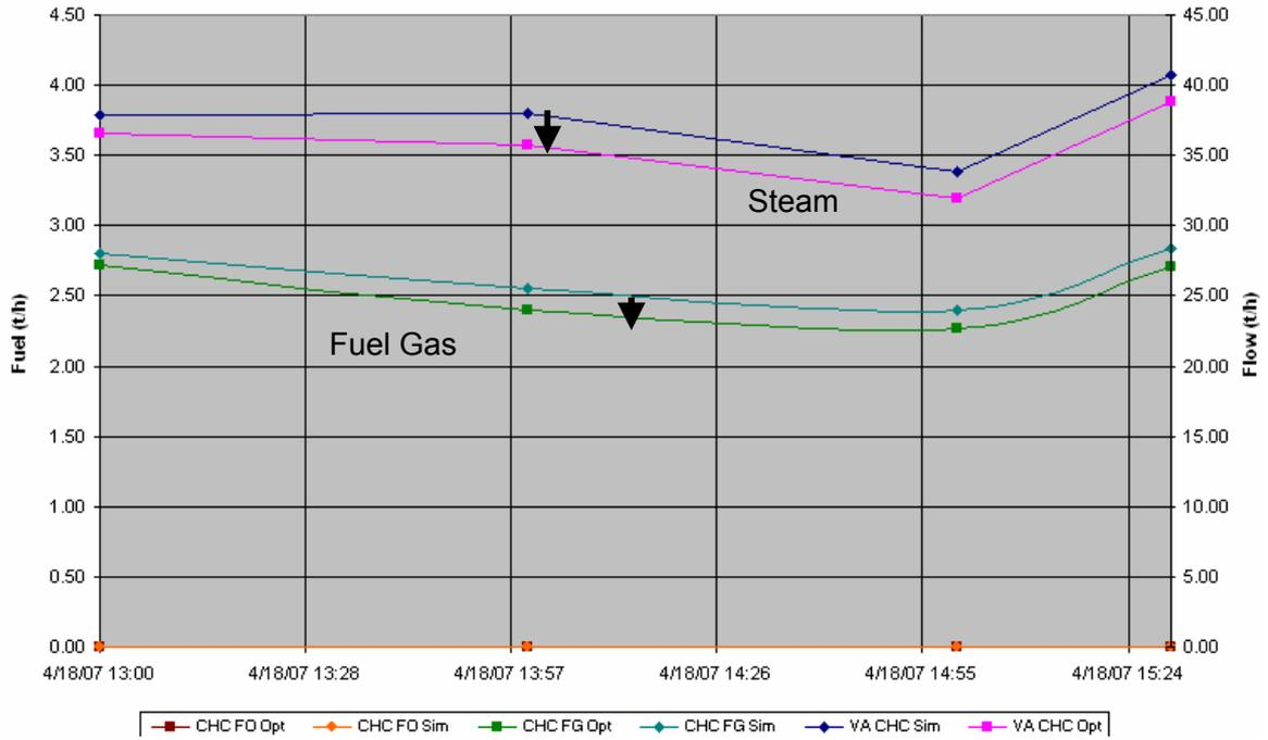
Boiler C (100% Fuel Gas): 2 t/h less of steam
