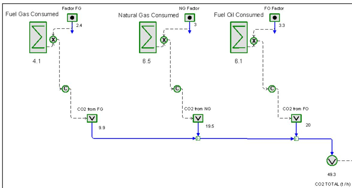
**Figure 3.** Details of the CO<sub>2</sub> emissions model differentiated by the type of Fuel
