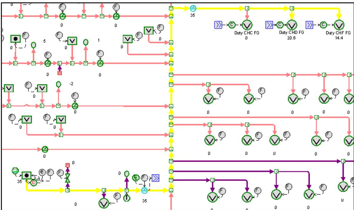
On the left, fuel gas suppliers are represented while on the right Fuel Gas consumers are displayed. The values indicate the corresponding change, expressed in MW, after the application of the recommendations (zero value means no change).
